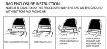
DEBRIS BAG FOLDING LABEL LOCATED ON BAG
